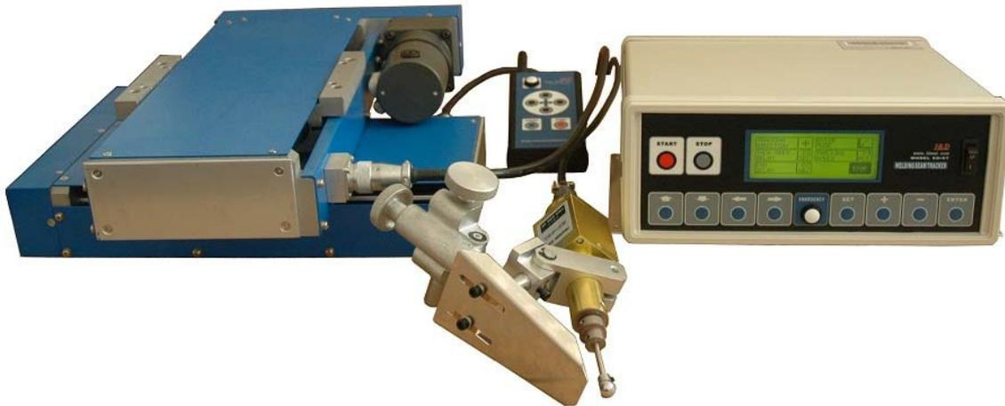
This ED-ST series welding Seam Tracker consists of sensor, control box and actuator (motorized slider), etc. Its working principle: data on welding face variation is collected by sensor touching work-piece, calculated by control system, and then distance between welding torch and work-piece would be adjusted accordingly when necessary by actuator, assuring welding quality.
