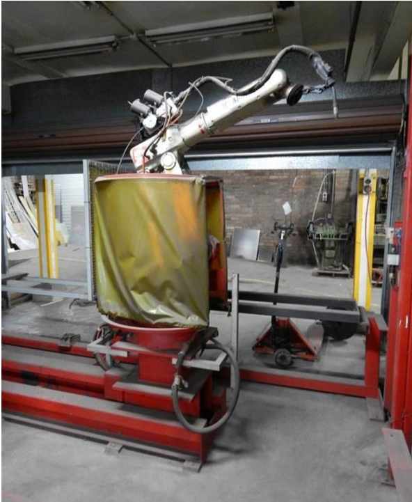
Robotic Welding Station, Yasnac ERC Model K10S comprising track mounted
