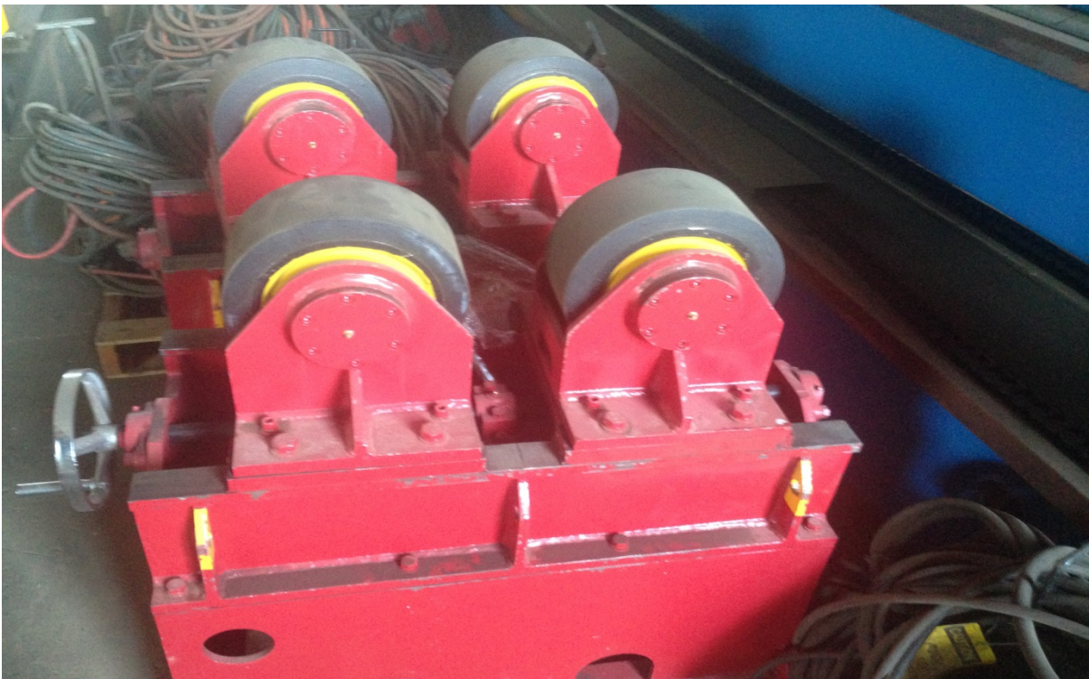
5 Ton capacity ideal for pipe spooling fabrication complete with idle rollers
